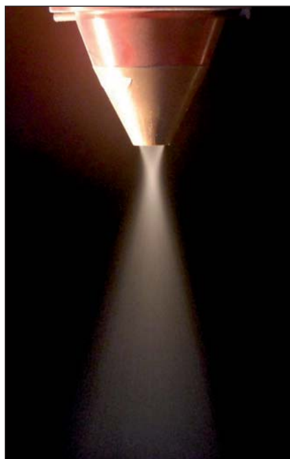
Focused free-flowing powder stream
