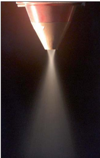
Focused free-flowing powder stream
