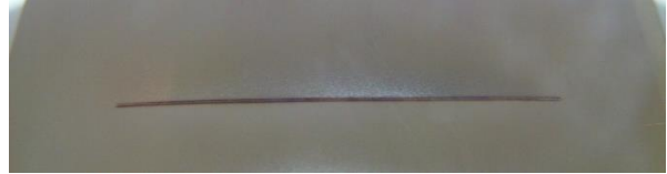
Figure 8: Welded test coupon (2 x 50 μm) with a weld path length of 30 mm without buckling
