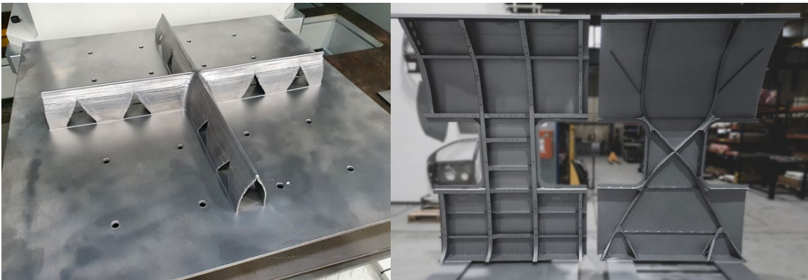
Figure 5 Left: Geometrical feature of the final part manufactured by wire-LMD. Right: Full demonstrator by powder-LMD manufactured at Photon AG
