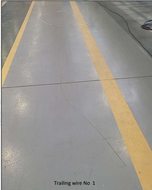
After wire straightening by a two plan seven roller wire straightener
