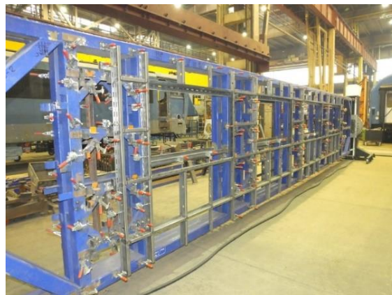
Figure 14 . Rotary side frame welding device (MÁV-VAGON, 2022)
