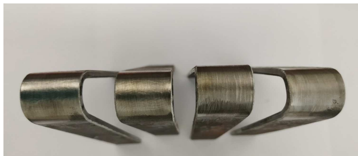
Fig10 Images of the bend test of the 3mm butt weld sample
