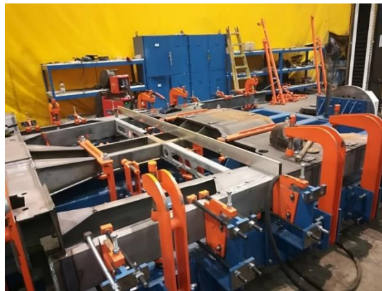
Figure 13. Chassis end assembly device (MÁV-VAGON, 2022)
