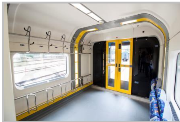
Figure 3. Bicycle storage room (MÁV-VAGON, 2022)
