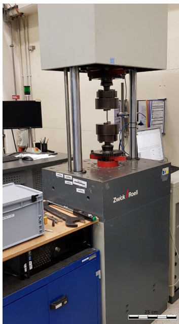
Figure 4: High-frequency pulsator ZWICK/ROELL HFP (left) and specimen for press-bolts M8 (right, top) and M10 (right, bottom)
