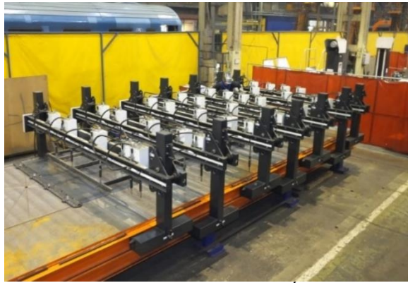
Figure 15. Side wall assembly device (MÁV-VAGON, 2022)
