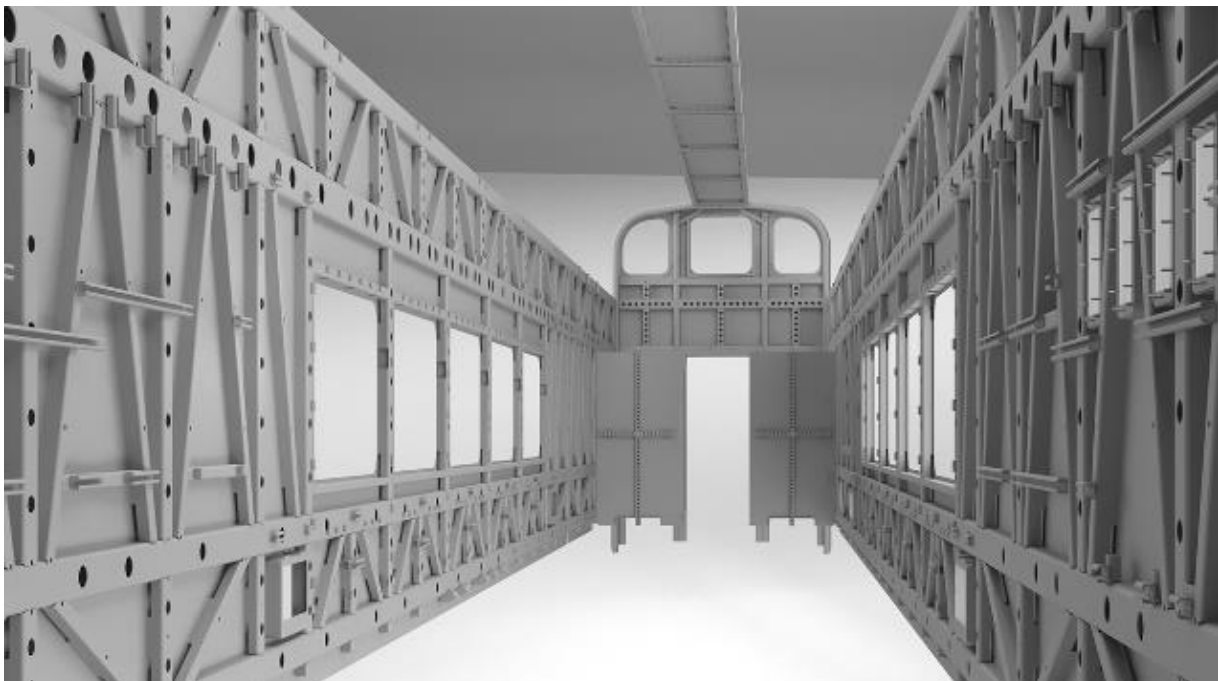
Fig. 1: Inner view of the parts manufactured by Photon for the Stadler Rocky Mountaineer (Copyright Photon)
