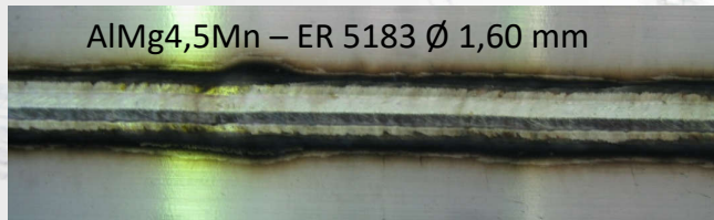
Welding from the drum with a guide pulley
