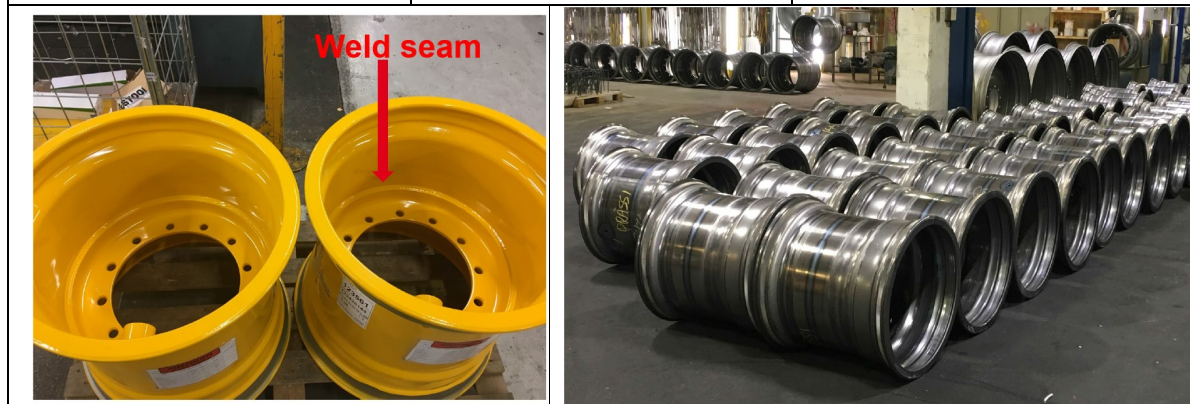
Figure 10: Welding of rims; material thickness: 8 mm, base metal: S235JR acc. to EN 10025
