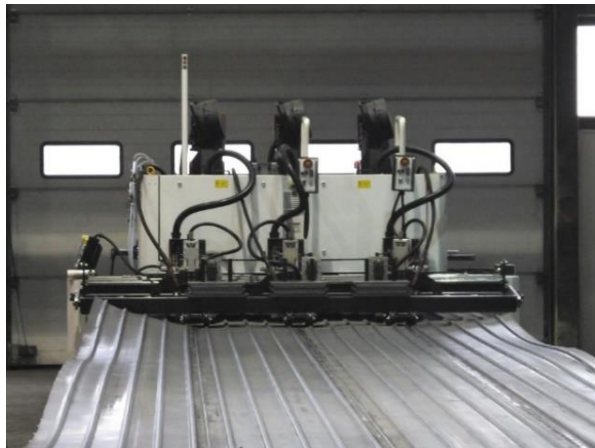
Figure 16. Roof plate welding equipment (MÁV-VAGON, 2022)
