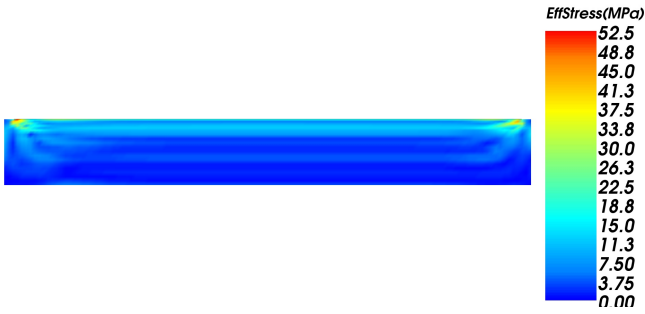
FIGURE 5: The effective or von Mises stress distribution is shown when the weld is at the end of the welding for Design A.
