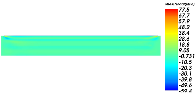
FIGURE 6: The longitudinal stress or \sigma_{xx} distribution is shown at the end of the welding for Design A.
