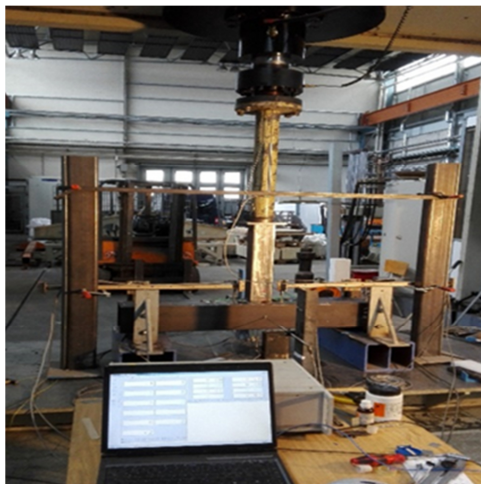
Figure 5: Compressive test configuration
